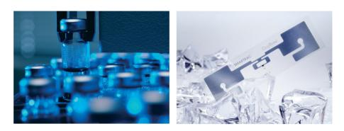
Temperature Sensor Dogbone is a general-purpose temperature sensor that is designed to work across a wide variety of materials, providing both good read distance and sensing performance.
