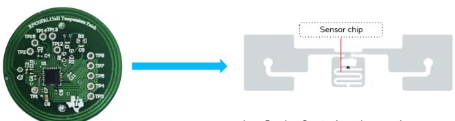
Avery Dennison Smartrac's passive sensor is a single-chip design that uses low-cost construction techniques, and requires no batteries and no maintenance. This results in a solution that costs a fraction of the price of traditional sensors, and its passive nature enables deployment in sensitive environments where an electric power source is not allowed.
